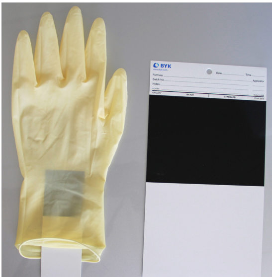
Picture 5: Sample preparation of a rubber glove for opacity check
