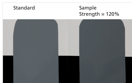
Picture 4: Drawdown of Standard/Sample with tinting strength
