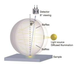
A sphere instrument may be operated under two different measurement conditions: **specular included (spin)** or **specular excluded (spex)**. In the "spin" mode, the total reflected light is measured. In the "spex" mode, a gloss trap is used to capture the directly reflected light (gloss). Color is measured independent of the sample's gloss or surface texture
