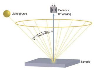
The 45/0 geometry simulates the normal condition used for color evaluation. For example, when we read a glossy magazine we position it to avoid the gloss from coming into our eye. A high gloss sample with the same pigmentation is visually judged darker by the eye when compared to a matte or structured sample.
