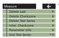
Press mode wheel to display a menu which allows deletion, interruption of a checkzone (=skip) or ending of a test series.
