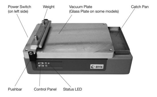
Some of the factors affecting the drawdown are the shear rate and the pressure placed on the applicator tool. The byko-drive employs a precise speed control along with a consistent weight to suit the particular material being applied.
