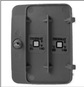
On the inside of the battery compartment lid are two thermo-sensitive stickers. They react at a exceeded temperature of 60°C (140°F) respectively 65°C (149°F). When these temperatures are exceeded, the color of the stickers turn to black. If the temperature has exceeded 65°C (149°F) please return the instrument to the manufacturer for verification.
