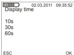
You can set the time interval after which the instrument shuts down automatically.
