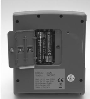
To operate the instrument, the battery compartment must be fitted with two 1.5-V AA(LR6) batteries.
