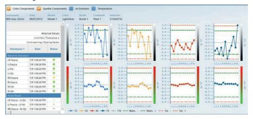
The scales to be shown in the graph can be selected with the icon **Graphs**. Select the required scales by using the **Arrow buttons**
