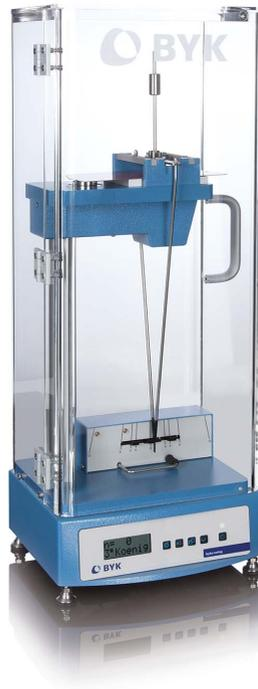
The **byko-swing** offers a fully automatic measurement mode - no manual interaction is required.
