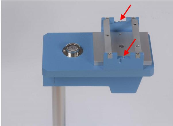
The marking arrow on the bar of the pendulum **must point to the front**.
