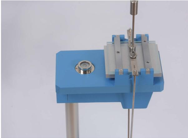
For periodical control of the instrument, it is recommended to measure **once a week** on the glass standard included in delivery.
