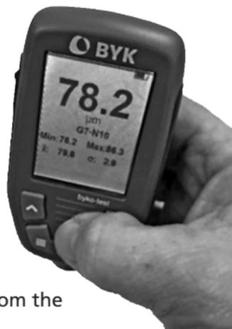
Press the instrument probe firmly against the surface to be measured. Remove from the surface and read the measurement directly on the screen. The backlight will turn off in 15 seconds, to restore the backlight simply press either the Up  $\wedge$  or Down  $\vee$  arrow buttons.
