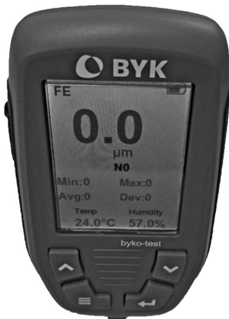
A full-color TFT screen is used to display the measurement, statistics, and environmental information as selected by the user.
