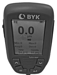
A full-color TFT screen is used to display the measurement, statistics, and environmental information as selected by the user.
